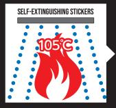
Automatic spraying of extinguishing agent with heat of 105°C.
